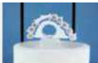
Correct position on the sintering tray
